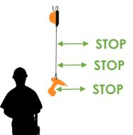
**2.** Tool stays automatically at a predefined position. This ensures a tool readiness for repeating assembly steps.
