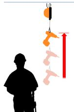
2. After work, the tool is automatically retracted to its initial position.
