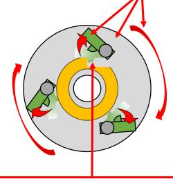
Due to the acceleration and the associated higher centrifugal force, the pins are pushed outwards and the ratchet lock is automatically released (unlocked).
